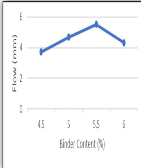
Upon examining the curves depicting the relationship between bitumen content (%) and stability (maximum value), unit weight (maximum value), and air voids (equivalent to 4% air voids), it was noted that the peak values for these parameters were all 5.5%. Consequently, the optimal bitumen content (OBC) was determined to be 5.5% based on the average value of the aforementioned three parameters.
