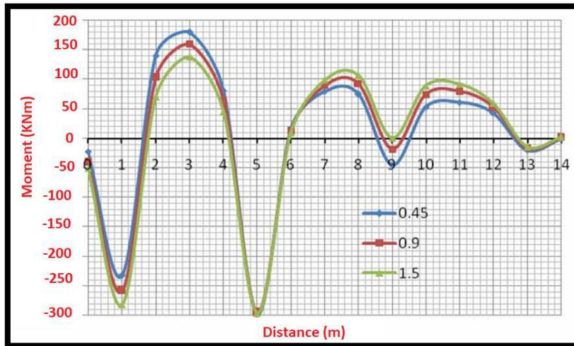
Figure -11, comparisons of raft thickness at Loading pattern III
