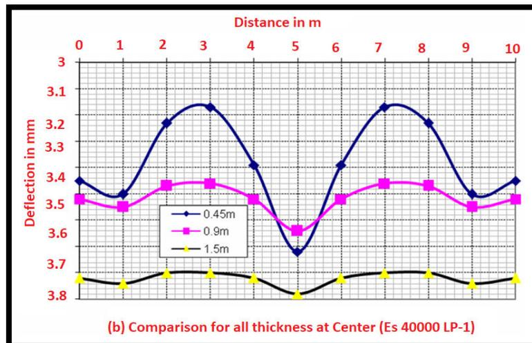
**Figure -6, Deflected shapes at Loading pattern -1**
