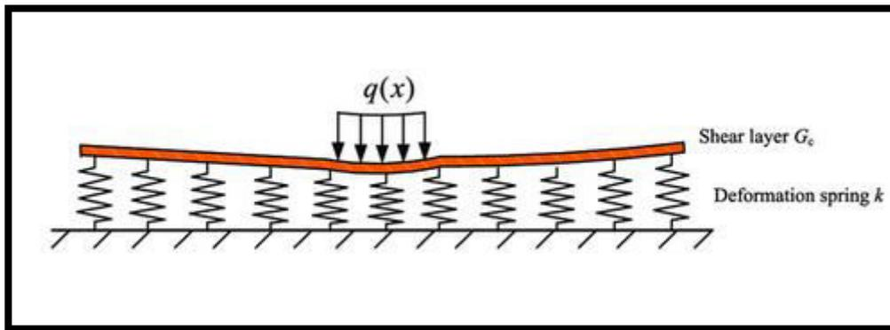
Figure -1, Pasternak foundation Model
