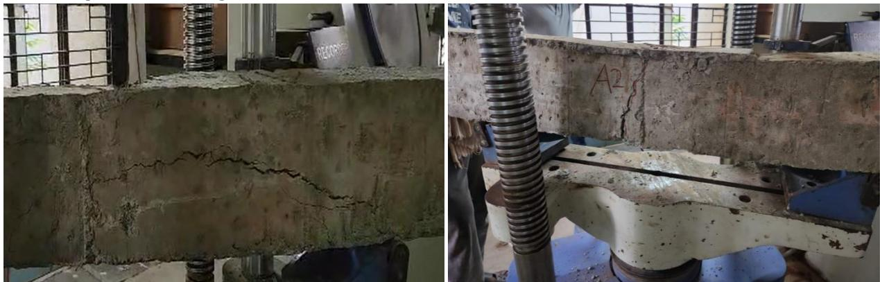
**Fig. 4** Failure and cracking pattern of beams
