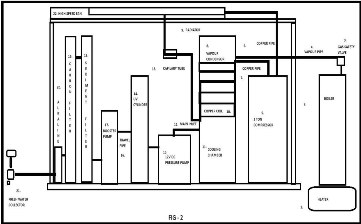
**Figure 3:** Schematic representations of the various components used in the desalination filter
