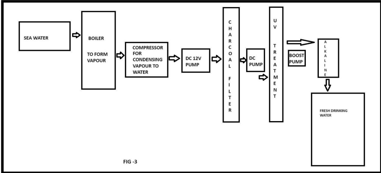
**Figure 4:** Block Diagram of the Filter
