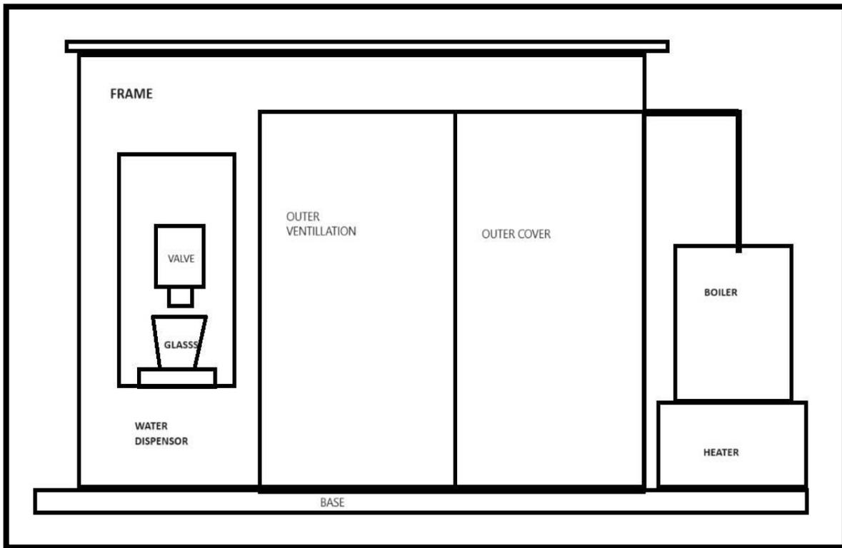
**Figure 2:** Side view of the Desalination Filter
