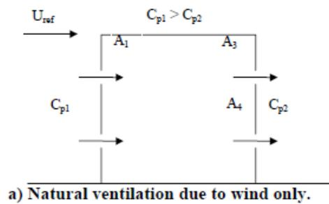
Figure 2: natural ventilation of a building by the dominant driving forces (Straw, 2000)
