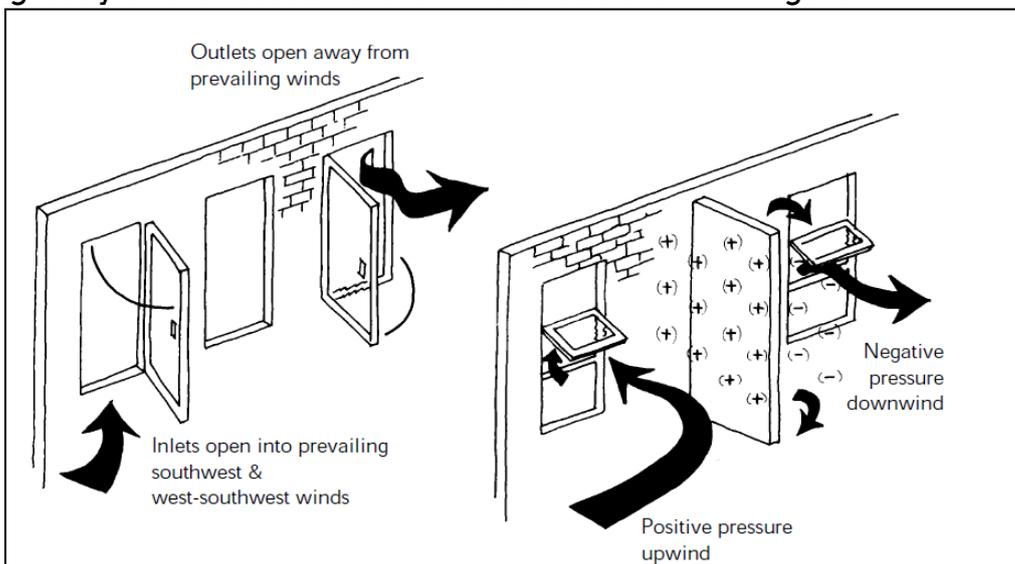
Figure 4: Orientation of Window to Prevailing Breeze (GBD, 1999)
