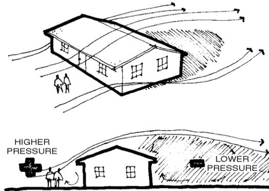
Figure 1: Aerodynamics around building (Evans, 2010)
